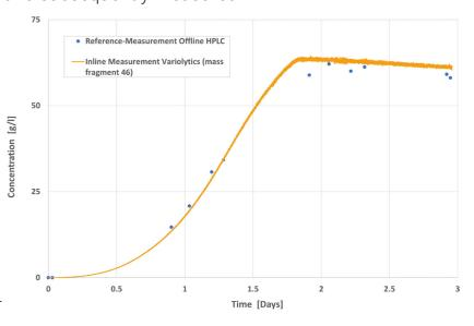
established analytical methods. The Variolytics measurement method has a lower time consumption, as no sampling and sample preparation is necessary. In addition, measurement is performed in real time so that the process can be directly controlled with the generated measurement data.
